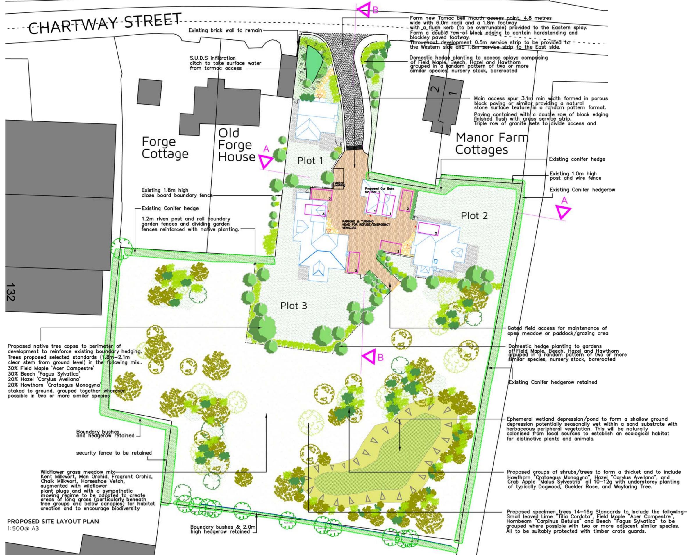
Form new Tarmac bell mouth access point, 4.8 metres wide with 6.0m radii and a 1.8m footway with a flush kerb (to be overrunable) provided to the Eastern spall. Form a double row of block edging to contain hardstanding and blockley paved footway. Throughout development 0.5m service strip to be provided to the Western side and 1.8m service strip to the East side.
