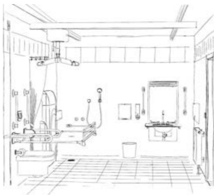
Community centre - Changing places toilet
