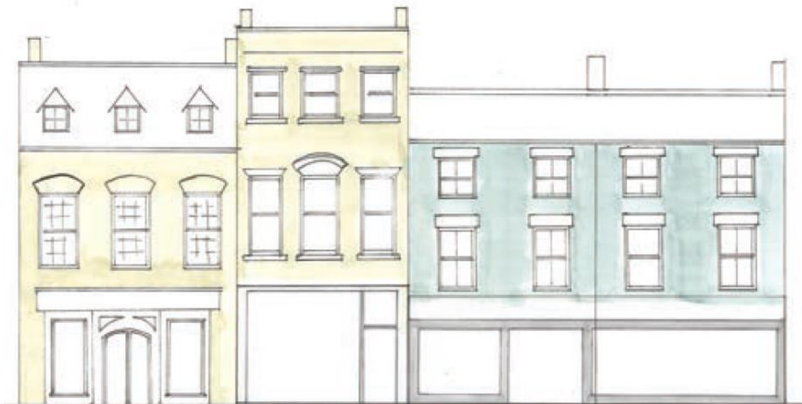
Figure 5 – poor street scene, with overlarge shop front and a combined shop front across two buildings.
