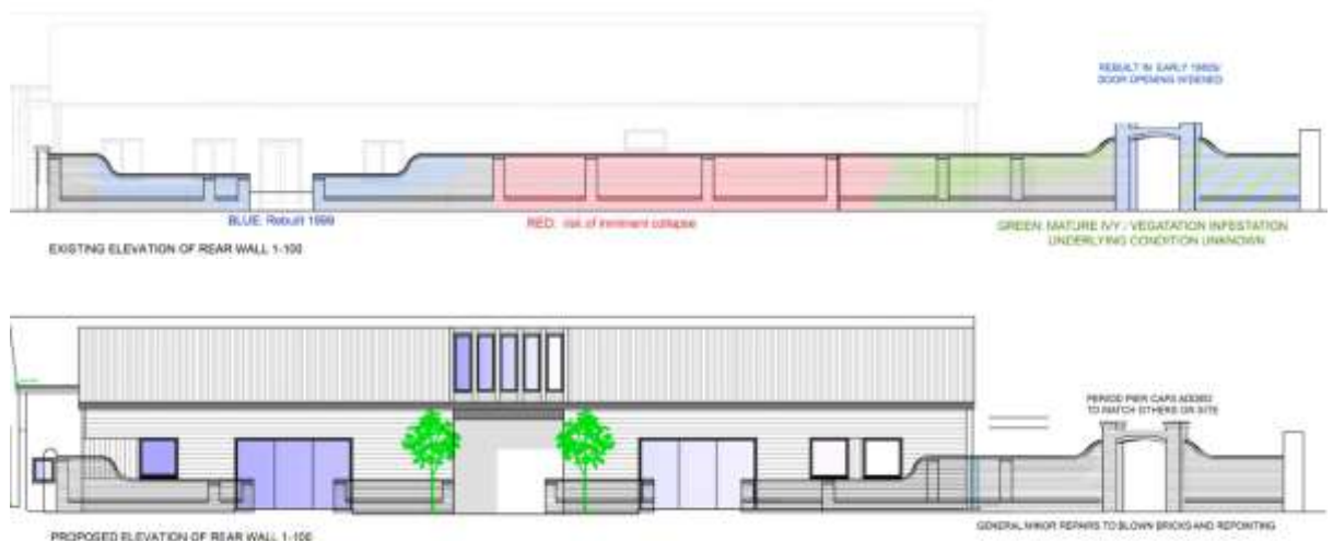
Figure 2 Works to the wall at the rear of the studio building
