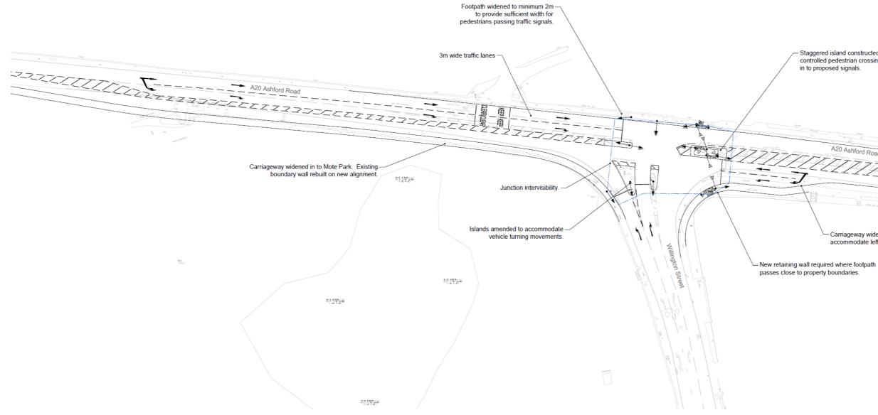
Staggered island constructed and new controlled pedestrian crossing integrated
