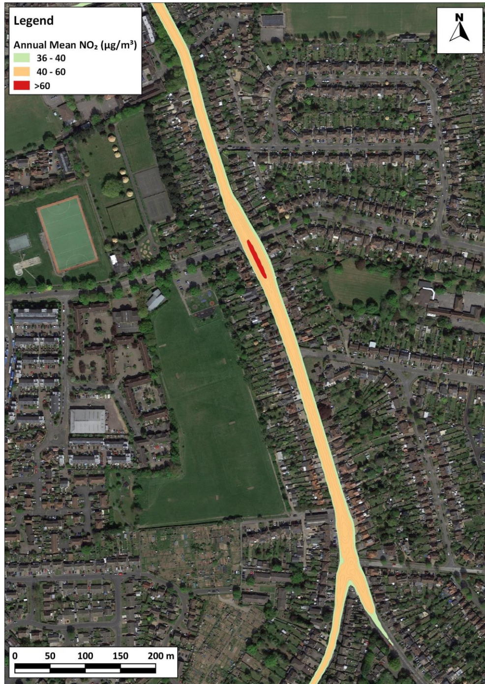
Figure 12: Contour Map of Modelled Annual Mean Nitrogen Dioxide Concentrations in 2019 Baseline along Loose Road
