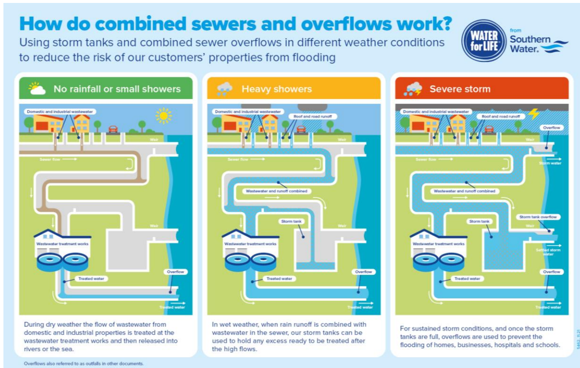
Figure 7: How do combined sewers and overflows work?
