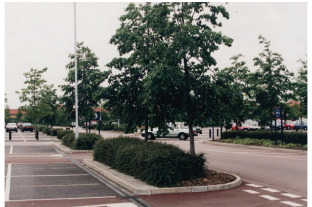
In intensively-used car parks small strips of paving adjacent to parking bays will prevent trampling of planting which results in bare patches
