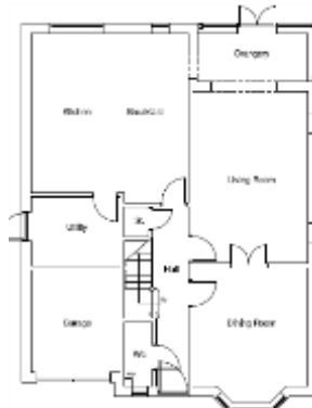
Layout Following Orangery Extension and garage alterations
