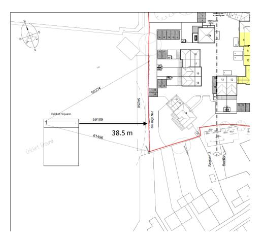
The above diagram illustrates the minimum measured distances from the edge of the cricket square to the proposed 8 m high netting. Note as this is a risk assessment the worst case scenarios are considered; consequently the shortest measured (and calculated) distance is used for the study.
