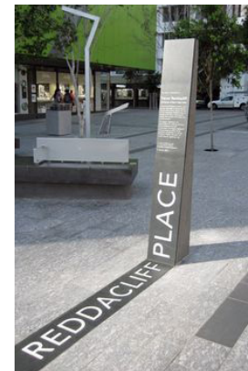
■ Bespoke wayfinding sign 2000mm height x 400mm width in steel, powder coated with bespoke lettering
