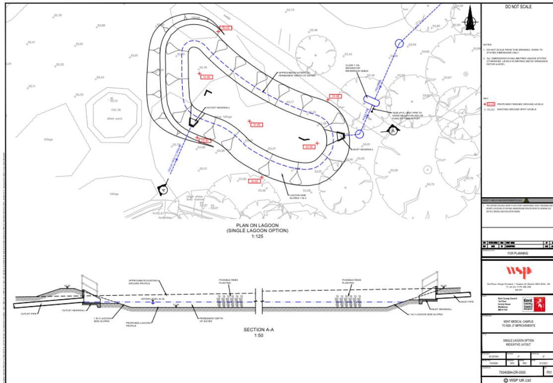
The lagoon would need to be of at least a similar size to the combined sizes of the current two lagoon option in order to provide sufficient attenuation storage volume. Entry and exit headwalls with associated safety fencing would also be required.
