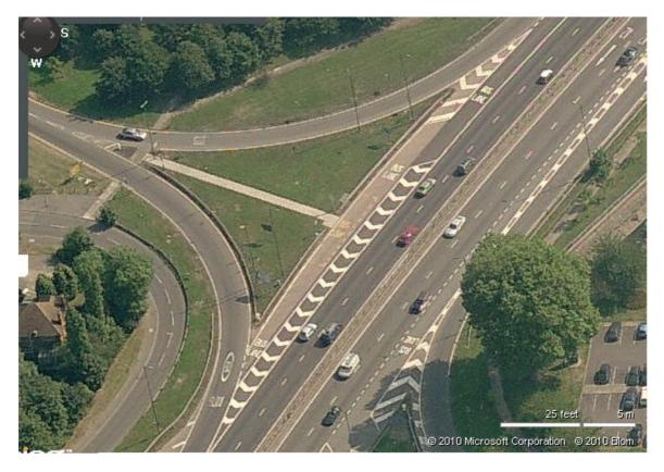
Option 3: build a new bus-stop layby at start of the acceleration lane from Cobtree Golf Course together with a bus-lane across the grass island at mouth of junction (likely to be in the region of £80K).
